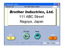
When the Print ID Label dialog box appears, check the stamp size, insert the appropriate ID label into the ID label slot of SC-2000USB, and then click the OK button.
